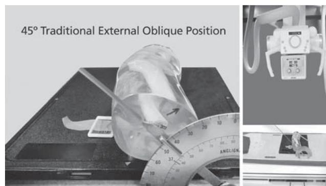
**Figure 2.** This setup demonstrates the traditional method of performing this study. The phantom was rotated laterally so the interepicondylar plane was at a 45° angle to the image receptor. The resulting image was used as a control image for comparison purposes.
