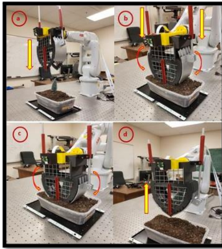
Fig. 9: Process of roguing the sample plant by prototype mechanism
