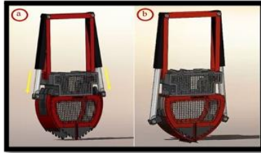
Fig. 7: Actuation of blades by hydraulic system in final design
