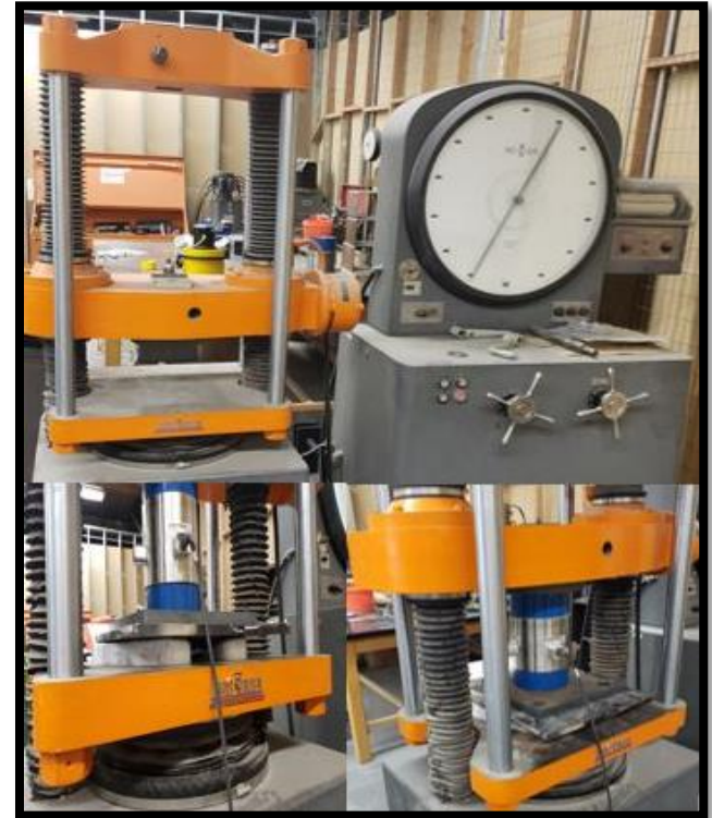
FIGURE 10: ELECTROMECHANICAL TENSILE & COMPRESSION TESTING MACHINE (TINIUS OLSEN) AND COMPRESSION LOAD SENSOR
