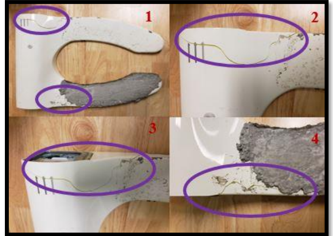
FIGURE 14: CRACK AND BREAKING POINTS IN THE SEAT #2
