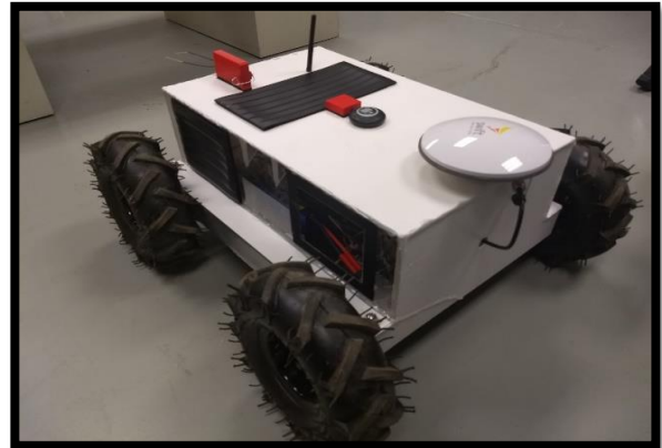
Fig. 10. Assembled and painted enclosure, placed on top of robot chassis.
