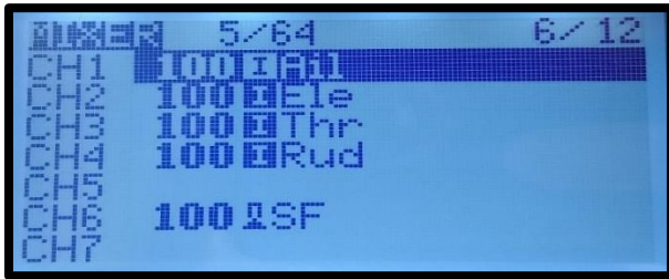
Fig. 6. Configuration for channel mixing on the Taranis transmitter. The switch used channel 6.
