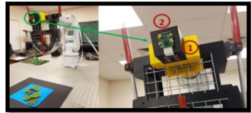
Fig. 5. The location of two cameras on a prototype of roguing mechanism. Camera 1 give us the top view of the plant and Camera 2 give us the front view of the plant.
